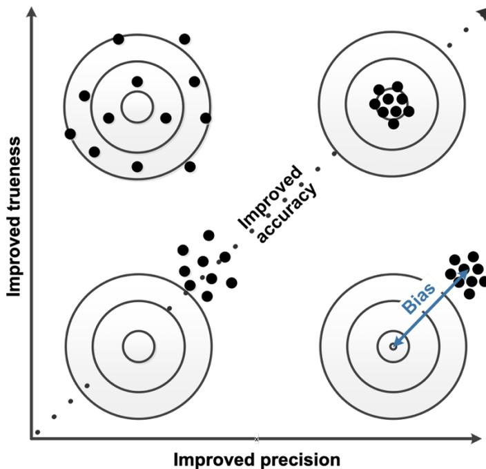
**Figure 3:** A graphical illustration of the meaning of trueness, precision, and their combination – accuracy.
