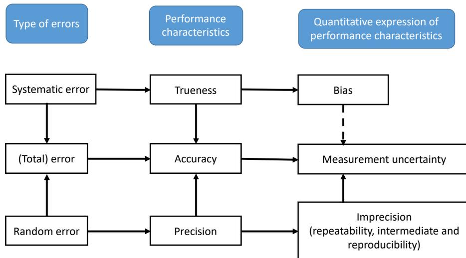
**Figure 2:** Concept diagram, adapted from Menditto et al. (13), explaining the relations between concepts describing, random and systematic errors as well as measurement uncertainty. The dotted line from bias to measurement uncertainty is to indicate that if bias can be estimated, it should be eliminated.
