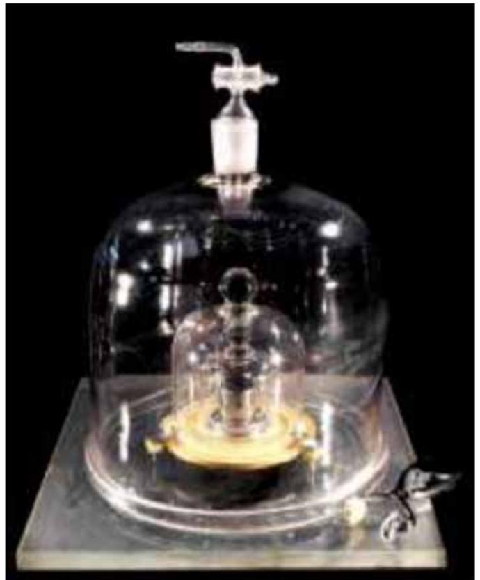
**Figure 1.** “The Kilo” – held under three vacuum seals at the International Bureau of Weights and Measures in Paris, France
